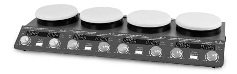
Thanks for choosing BT Lab Systems' BT1024 Hot Plate Stirrer, Multi position (4 positions) Individually Controlled. This operation manual describes the function and operation of the instrument. In order to use the instrument properly, please read this manual carefully.
